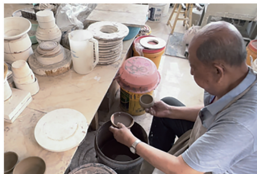
图 16 内部上釉 Figure 16 Internal glazing
